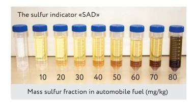
The result of indicator using is changing color of substance that depends of total sulfur content in automobile fuel.
