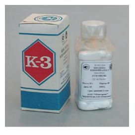
**IT IS APPLIED** in fuel and energy complex, coal, petrochemical industry, when calibrating and verifying the combustion bomb calorimeters, performs functions of the working standard.
