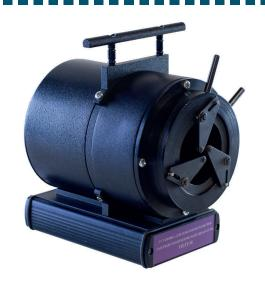
The installation УПЛТ-M is **DESIGNED FOR** reproducing, storing and transmitting of the unit of the average power and density power of the continuous and pulse-modulated optic emission, calibration and verification of integrated and autonomous photometers for laser medical equipment and laser therapeutical, surgical and therapeutical equipment.
